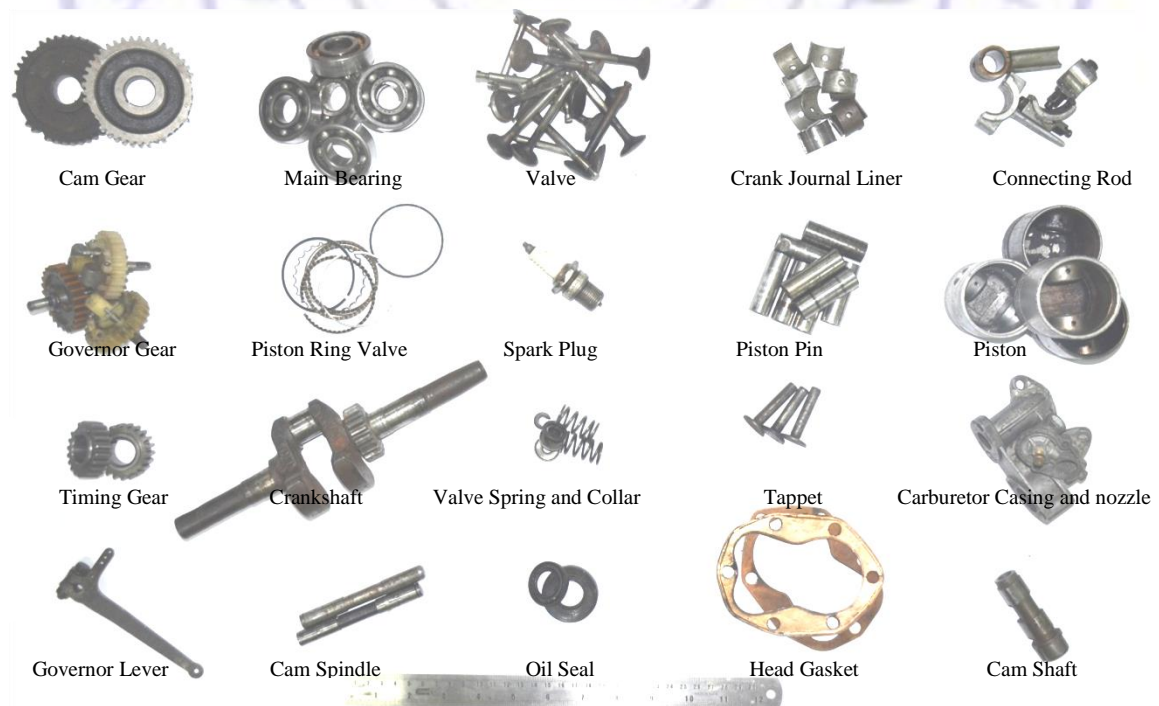
Figure 3.4: Samples Failed in the Field
